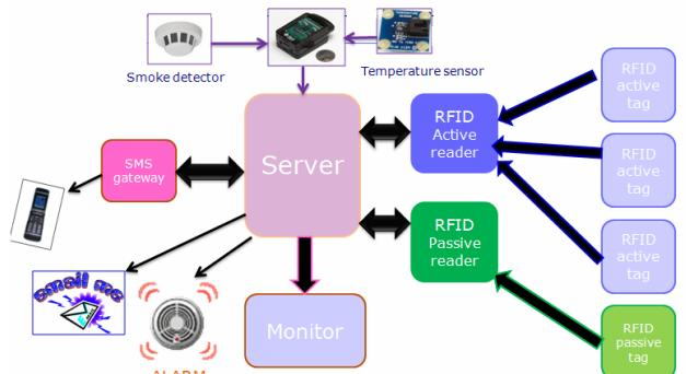
Fig. 2. Logical system architecture
