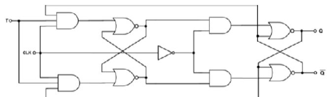
Figure 2: A T flip flop based on cross-coupled NOR gates.
