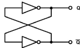
Figure 1: A bistable circuit constructed with cross-coupled inverters
