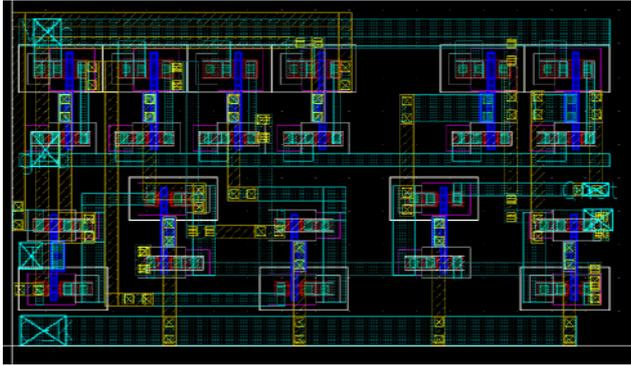
Figure 9: Proposed CMOS T flip flop layout.
