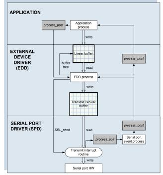
Fig. 1. Data flow from the application to external device
