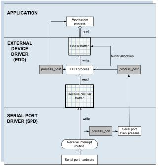
Fig. 2. Data flow from external device to the application
