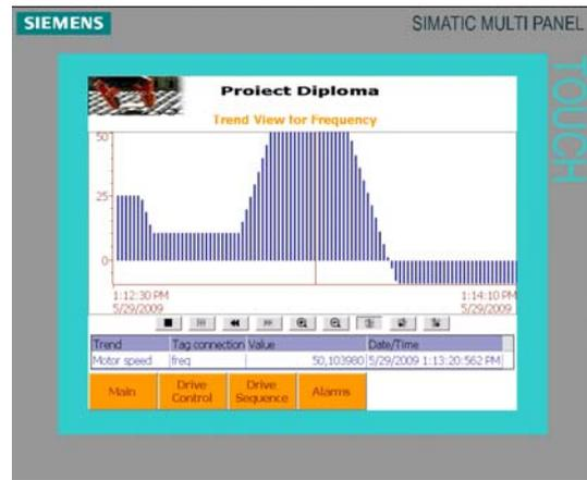
Fig. 8. Trend view for inverter frequency.
