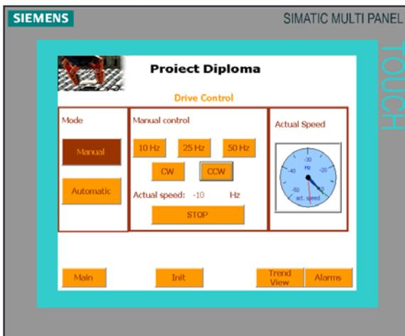
Fig. 6. Manual drive control mode.
