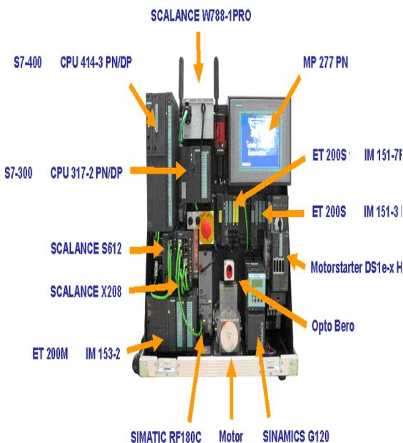
Fig. 1. SCADA – TIA Democase setup.
