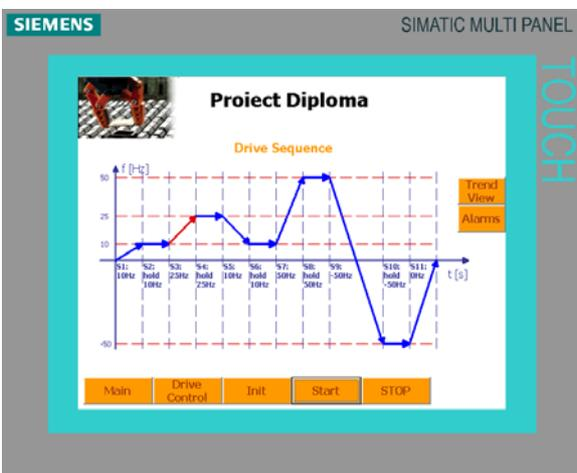
Fig. 7. Auto drive control mode-reference sequence.
