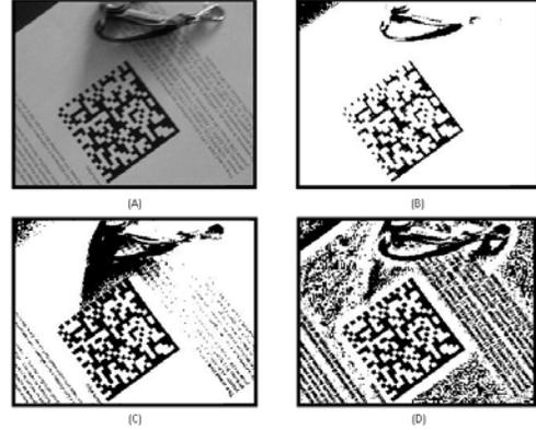
Fig. 2. (a) Original grayscale image (b) Histogram thresholding (c) Scan-line adaptive (d) Local adaptive
