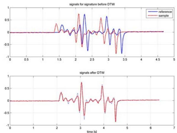
Fig. 3 time series for same writer recorded with input device writing two signatures before and after DTW.
