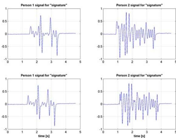
Fig. 2 Typical output of time series for same (columns) and different writers (rows) recorded with input device writing two signatures.
