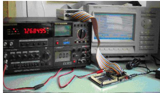
(a) Pulse generator and logic analyzer connected to the CYPRESS board with the programmed CPLD
