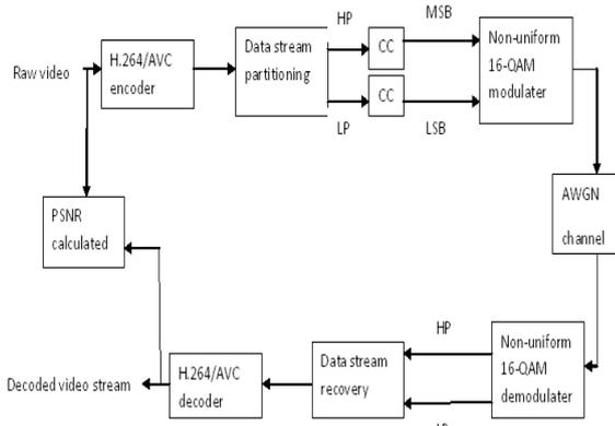
Figure 4. Block diagram of the proposed UEP scheme.
