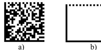
Fig.2, a) DataMatrix; b) Finder and timing pattern
