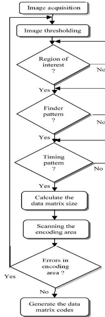
Fig.4, Process diagram
