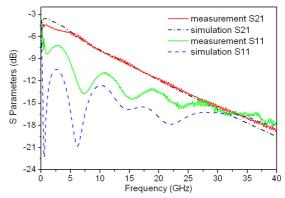
Fig. 3. Simulation and measurement results of a GCPW-MS-GCPW transition with rectangular stubs on SU8 resin with 370-nm aluminum metallization.
