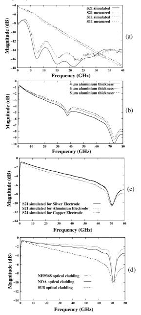
Fig. 4. S-parameters of a transition with CPW pads on 8μm thick SU8 (except d). (a) 370-nm thick aluminum metallization and L<sub>2</sub>=1 mm; (b) different thicknesses of aluminum metallization and L<sub>2</sub>=2 mm; (c) different electrode metals and L<sub>2</sub>=1 mm; (d) different substrate materials with 6-μm silver metallization and L<sub>2</sub>=1 mm.
