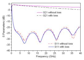
Fig. 2. Simulation results of a transition on SU8 with and without taking into account the dielectric losses, the aluminum thickness is assumed to be equal to  $4 \mu m$ .
