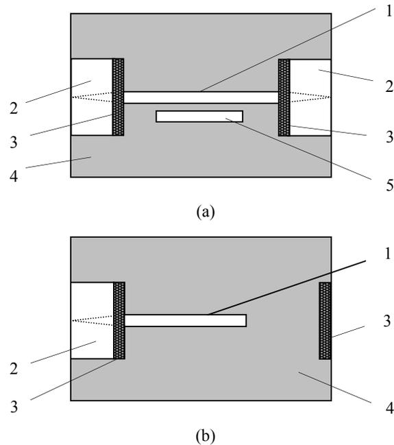
Fig. 1: The top views of the image guide structures. (a) coupled IG structure; (b) single open ended IG. 1 – IG; 2 – rectangular waveguide to IG transition; 3 – absorbing plates; 4 – metal plate; 5 – secondary IG.
