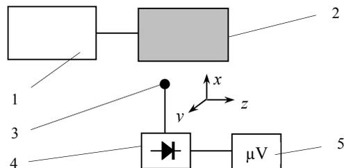
Fig. 3: The experimental setup. 1 – generator; 2 – the structure under investigation; 3 – the movable electric probe; 4 – detector; 5 – microvoltmeter.
