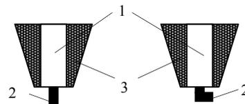
Fig. 2: The electric probes for  $E_y$  component (left) and  $E_x$  and  $E_z$  components (right). 1 – semi-rigid coaxial cable; 2 – inner conductor; 3 – absorbing coating.
