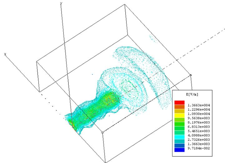
Fig. 5: Simulated distribution of the magnitude of the electric field at 33 GHz.
