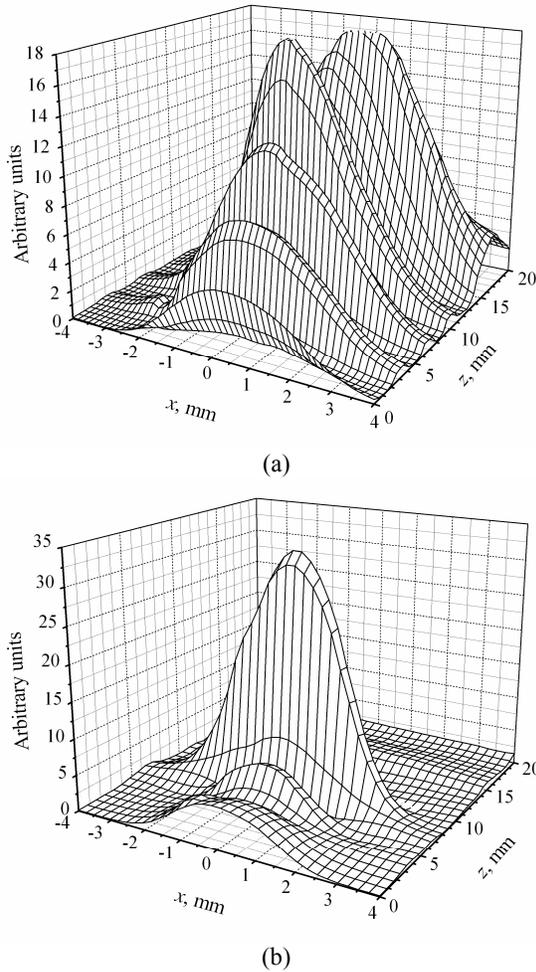
Fig. 4: The measured distributions of the  $E_x$  (a) and  $E_z$  (b) components.
