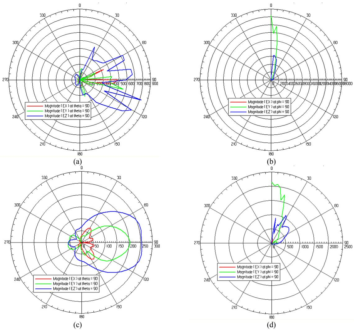
Fig. 6: Simulated polar diagrams for the near field at a frequency 33 GHz.
