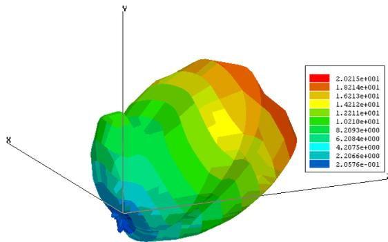
Fig. 8: Simulated 3D antenna directivity pattern at 33 GHz.
