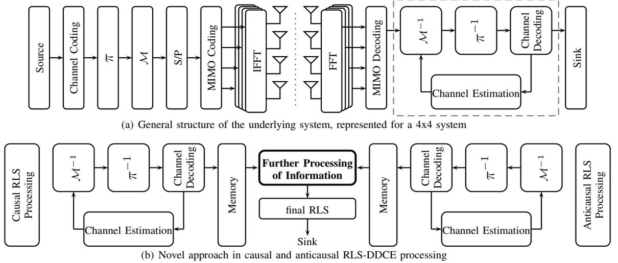
Fig. 1. Illustration of the system structure in Figure 1(a) and our proposed improvement, implemented on the receiver side of the system, in Fig. 1(b)
