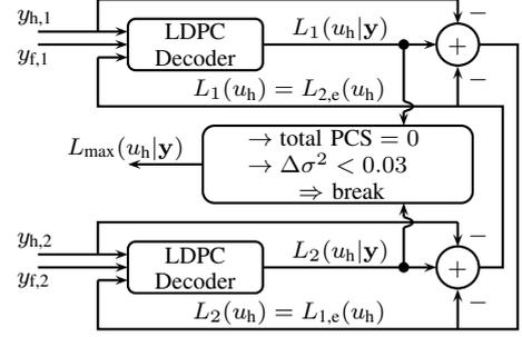
Fig. 3. Modified Turbo Principle
