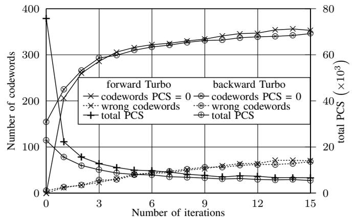
Fig. 5. Iterative behavior of the Turbo principle showing the number of correct codewords, wrong codewords and total PCS for the forward and backward Turbo iteration, at a SNR of 18 dB and 8.33 m/s
