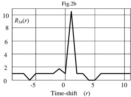
Fig. 2. The CCF of the sequences  $\{\zeta_2(j)\}_{j=0}^{10}$  and  $\{\zeta_6(j)\}_{j=0}^{10}$  (a), and sequences  $\{\zeta_3(j)\}_{j=0}^{10}$  and  $\{\zeta_4(j)\}_{j=0}^{10}$  (b).
