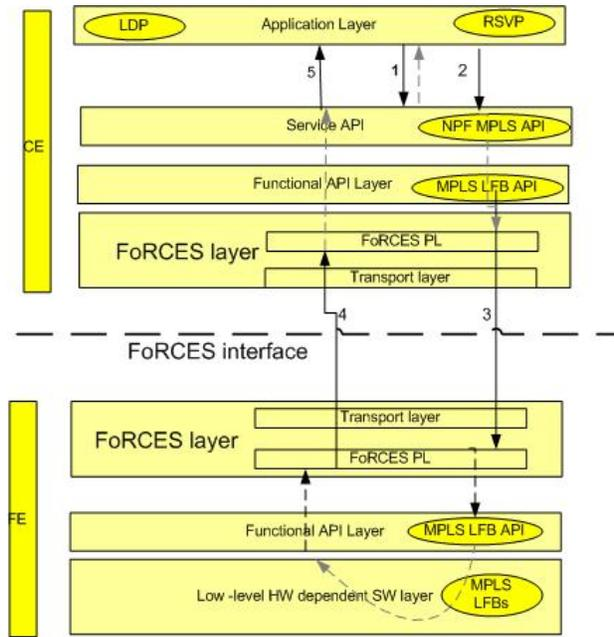
Fig. 3. Message flow: LSP creation in a distributed router.
