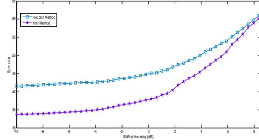
Fig.3. sum rate of PUs for two different methods of power allocation for selected subcarriers.
