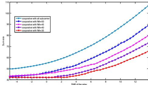
Fig.2. achieve rate of primary users for different numbers of selected subcarriers.
