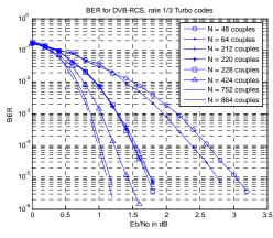
Fig. 3. Influence of block size on the BER performance of the DVB-RCS turbo code.
