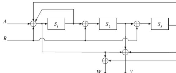
Fig. 2. Duobinary CRSC constituent encoder used by DVB-RCS.
