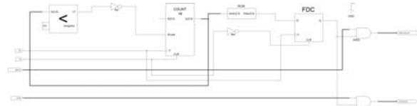
Fig. 7. RTL schematic of the puncture block
