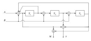
Fig. 2. Duobinary CRSC constituent encoder used by DVB-RCS.
