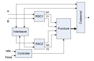
Fig. 1. Block diagram of DVB-RCS Turbo encoder.
