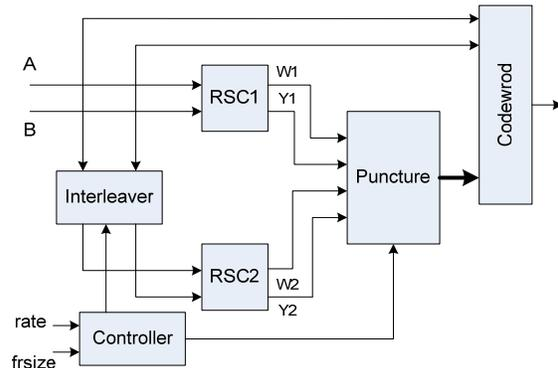
Fig. 1. Block diagram of DVB-RCS Turbo encoder.
