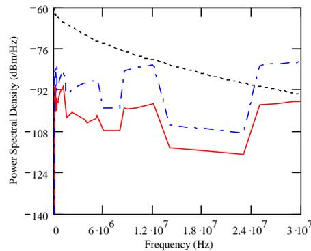
Fig. 3. Power spect. dens. of total noise for the real-case assumption
