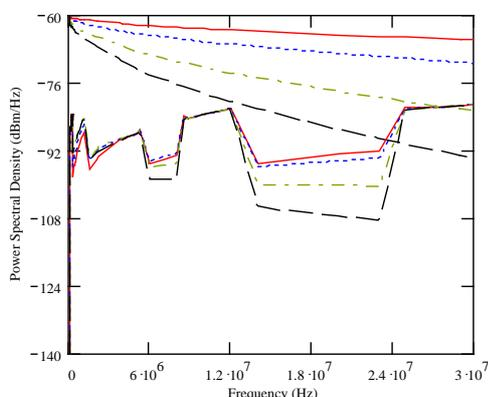
Fig.6. Power spect. dens. of total noise for diff. lengths-twisted pairs.
