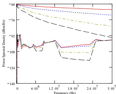
Fig.5. Power spect. dens. of total noise for diff. lengths-quad cables.
