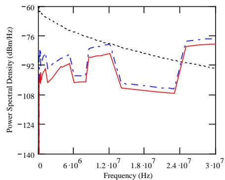
Fig. 4. Power spect. dens. of total noise for the bad-case assumption.
