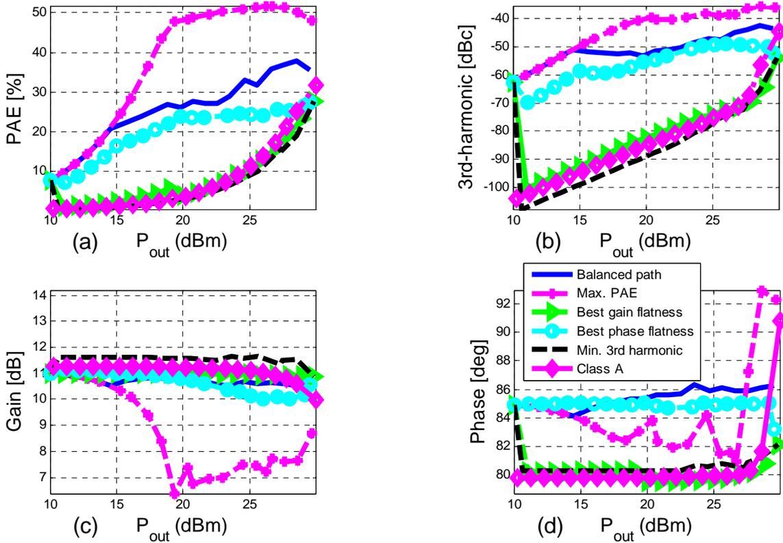
Figure 6. Results for the DB paths. (a) PAE (b) 3<sup>rd</sup> harmonic (c) Gain (d) Output phase
