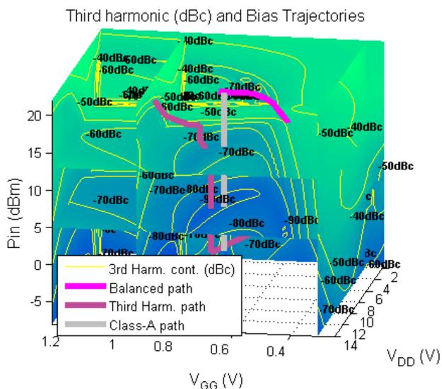
Figure 5. Third harmonic slices and contours with bias trajectories for balanced linearity/efficiency, minimum 3<sup>rd</sup> harmonic and class-A operation.
