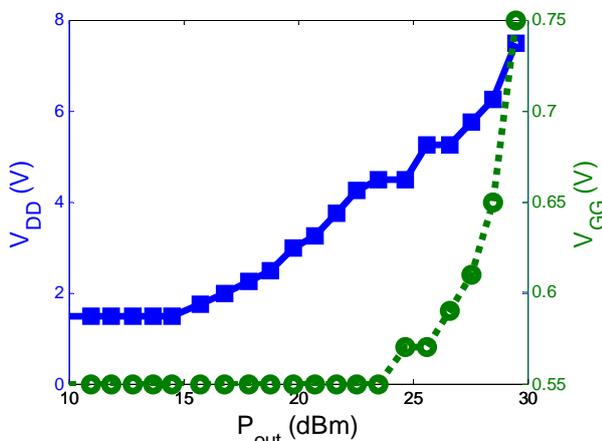
Figure 8. Bias as a function of output power for the balanced path.
