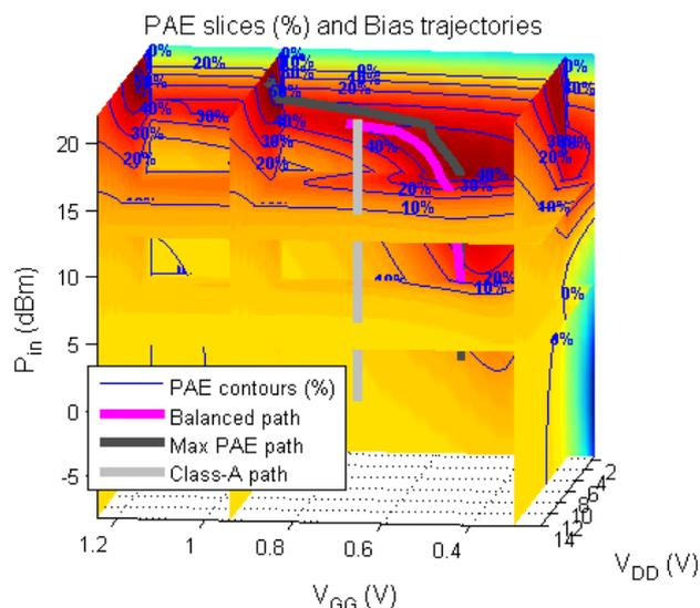
Figure 2. PAE and Pout slices and contours with bias trajectories for balanced linearity/efficiency, maximum PAE and class-A operation.
