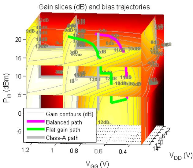
Figure 3. Gain slices and contours with trajectories for balanced linearity/efficiency, flat gain and class-A operation.
