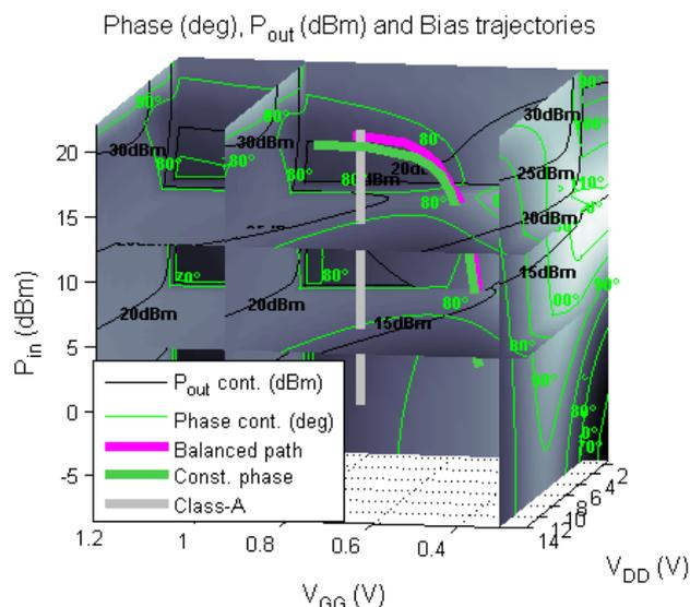
Figure 4. Phase and Pout slices and contours with bias trajectories for balanced linearity/efficiency, constant phase and class-A operation.
