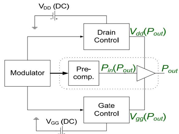
Figure 1. Simplified block diagram of the Dynamic Biasing system for class-A/AB amplifier enhancement.
