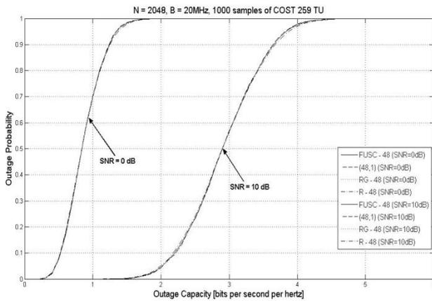
Figure 2. Outage Probability versus Outage Capacity for SNR=0 dB and SNR=10 dB
