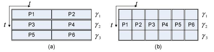
Fig. 2. Video transmission (a) not using diversity (b) using diversity
