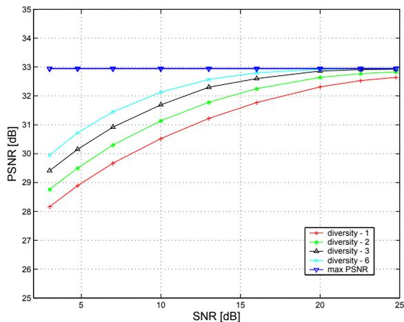
Fig. 5. PSNR in terms of average channel SNR
