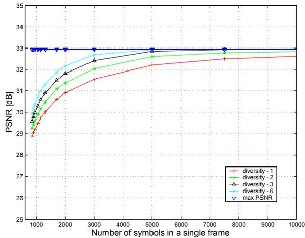
Fig. 4. PSNR in terms of number of available symbols in a single frame
