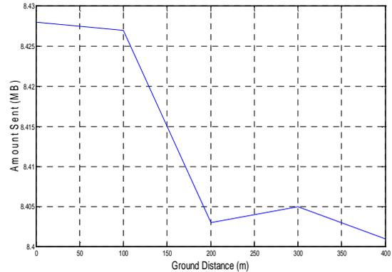
Figure 7: Amount of data sent on the uplink v/s ground distance for 802.11a 54Mbps
