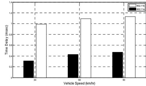
Figure 4: Comparison between 802.11a and 802.11b in terms of end-end delay at different speeds
