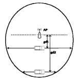
Figure 6: A larger Ground Distance results in a smaller connection time
