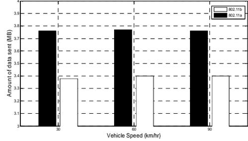
Figure 3: Comparison in terms of amount of data sent by 802.11a and 802.11b at different speeds
