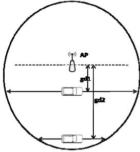
Figure 6: A larger Ground Distance results in a smaller connection time
