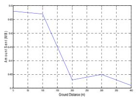
Figure 7: Amount of data sent on the uplink v/s ground distance for 802.11a 54Mbps
