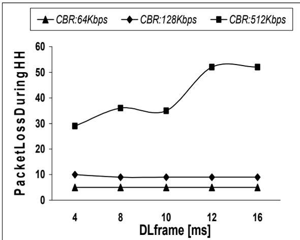
Fig. 2. Packet loss during the HH procedure for CBR applications: BS is empty
