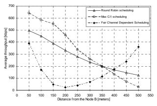
Fig. 2. Average throughput of the simulated mobile users
