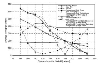
Fig. 4. Average throughput of all 14 packet schedulers using CAT 10 UEs
