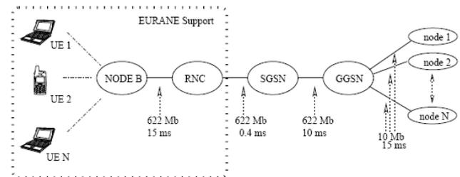
Fig. 1. Topology used in simulation
