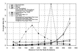
Fig. 5. Average delay of all 14 packet schedulers using CAT 10 UEs
