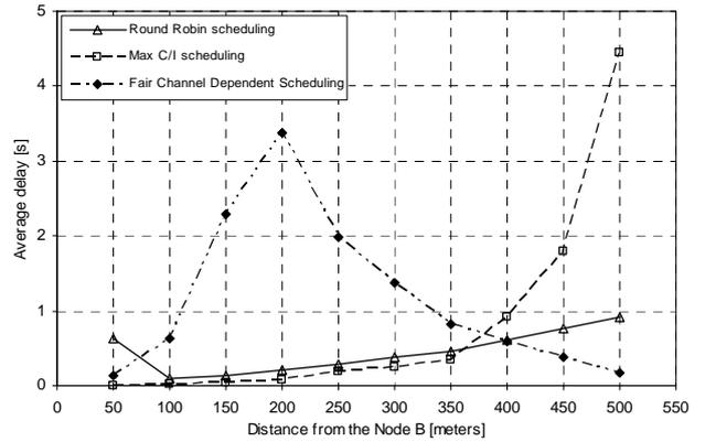
Fig. 3. Average delay of the simulated mobile users
