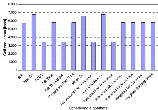
Fig. 6. Overall cell throughput for different Scheduling Algorithms
