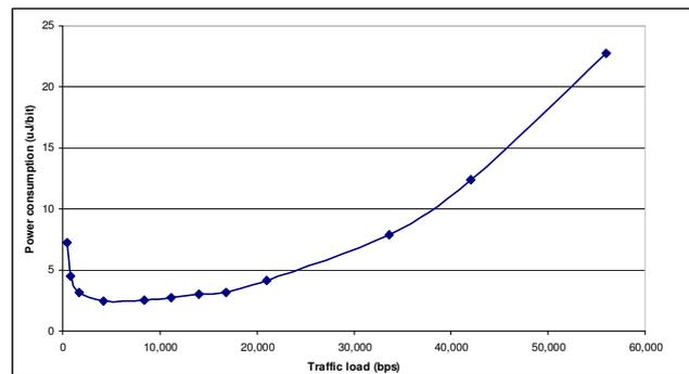
Figure 6. Energy consumption per transferred bit
