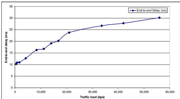
Figure 5. End-to-end delay of received packets
