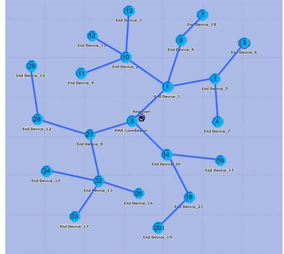
Figure 3. Cluster-tree topology of self formed network
