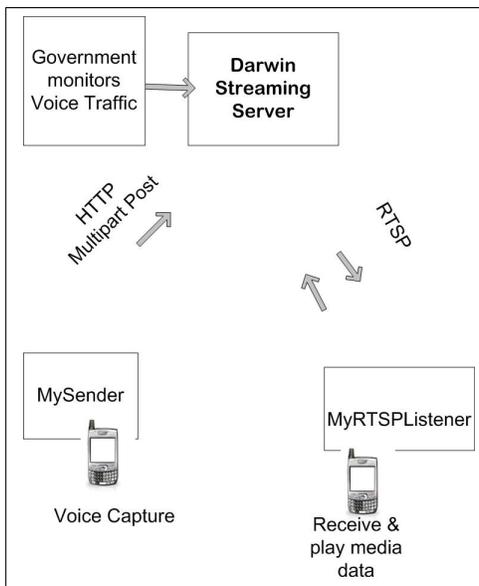
Figure 7: RTP based Government Controlled Mobile VOIP.
