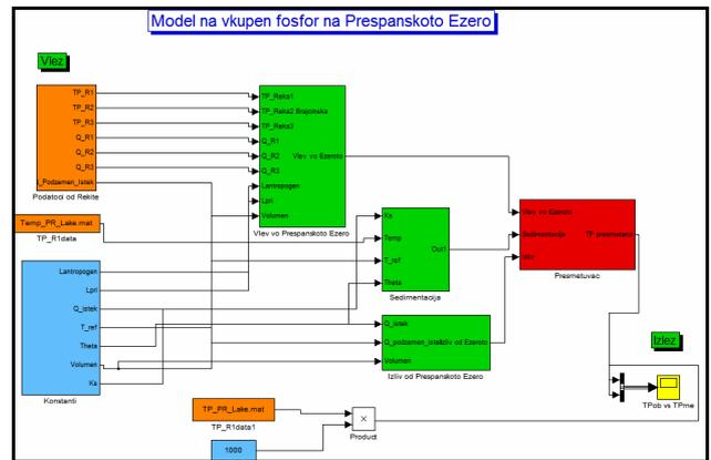
Fig. 2 -The TP model of the Lake Prespa in Matlab Simulink
