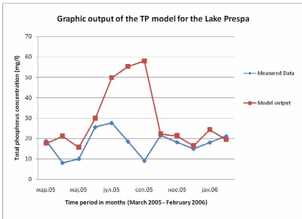
Fig. 3 -Graphic output of the TP model of the Lake Prespa for 12 months period
