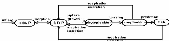
Fig. 1 -Conceptual diagram showing the components of the model as a part of the phosphorous cycle
