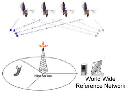
Fig. 3. A-GNSS Based Positioning
