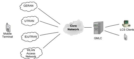
Fig. 1. General LCS Architecture in 3GPP Rel 9
