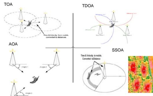
Fig. 2. Mobile Network Based Positioning Methodologies
