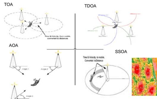
Fig. 2. Mobile Network Based Positioning Methodologies
